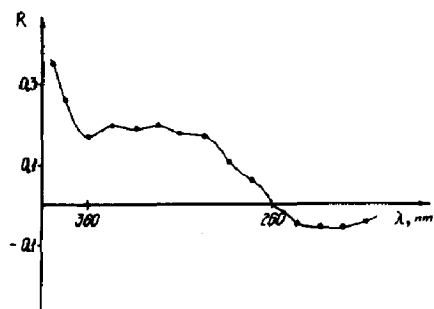
Fig. 8. Excitation anisotropy spectrum of an n -pentane solution of IV at 163 K.
